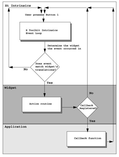
Figure 2-3: Event handling using action routines and callbacks
