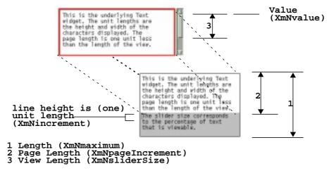
Figure 10-4: Conceptual relationship between a ScrollBar and the object that it scrolls
