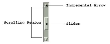
Figure 10-3: Elements of a ScrollBar
