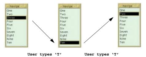
Figure 13-6: XmNmatchBehavior set to XmQUICK\_NAVIGATE
