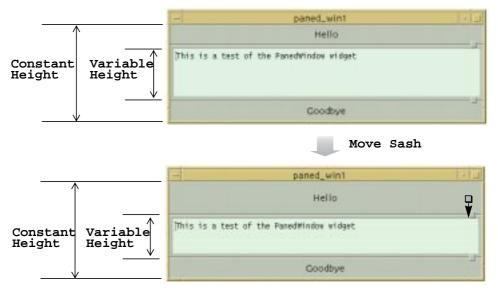
Figure 8-21 shows how the PanedWindow behaves when a child is resized using the Sash.
