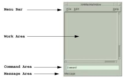
Figure 3-19: Recommended layout for MainWindow widget
