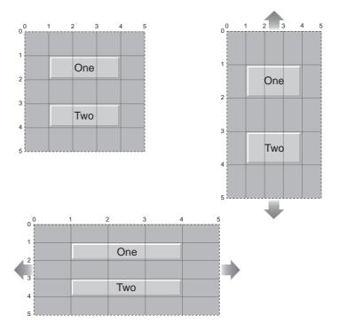
Figure 8-11: Form with XmNfractionBase set to 5
