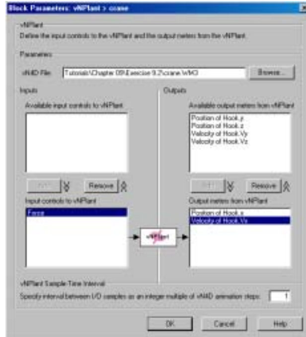
Figure 9-16 Block Parameters for the Crane model
